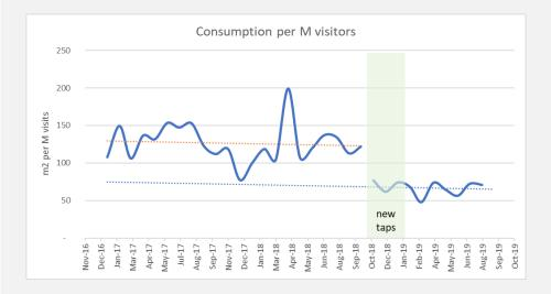
The graph displays the trend over time, based on the monthly potable water readings for the WC blocks where aerators were added. Significant improvements are evident from October-December 2018, coinciding with the installation of the new aerators.
